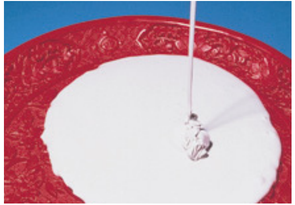
RTV silicone rubber flows easily into the tiniest of recesses.
