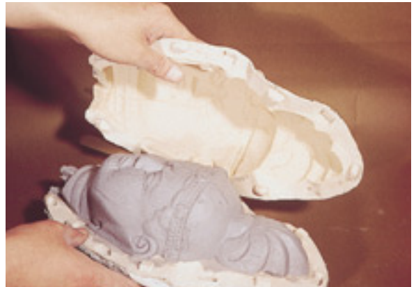
Making a mold of a sculpture using the lamination method
